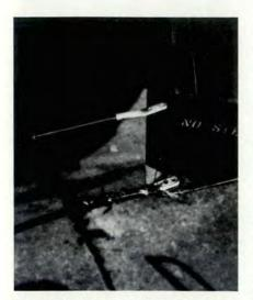
Designed to dissipate static buildup on aircraft, these "whiskers" were unable to handle the tremendous surge of a lightning strike.
